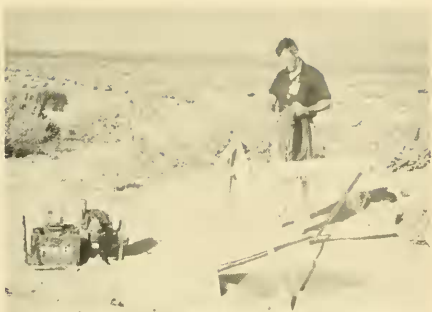
Fig. 3. Generator-operated, 40-watt ultraviolet light-trap supported on folding wooden legs. The shallow depression beneath was formed with a shovel, lined with a plastic sheet, and filled with detergent water.
